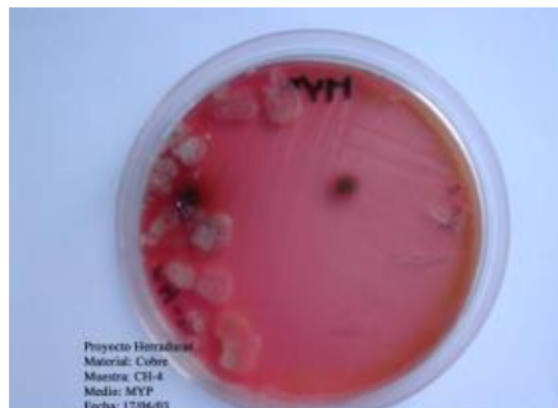
Photo 1. Sample CH-4. COPPER Horseshoe in MYP medium for detection of Bacillus sp
