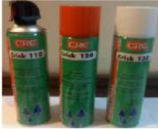
Figure 2: Kit of three aerosols. Cleaner (Crick 110), Penetrator (Crick 120) and Developer (Crick 130).
