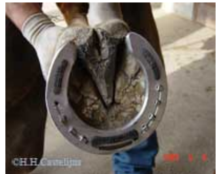
Fig 10: Alu gomma by Colleoni; the inserts are polyurethane
