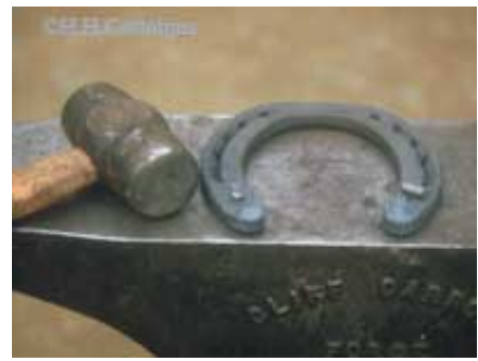
Fig 8: Widia (hard steel), antislip cones
